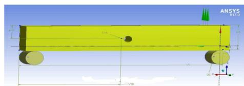
**Figure 11: RC Beam Having 265mm Depth with a Central Circular Opening**
